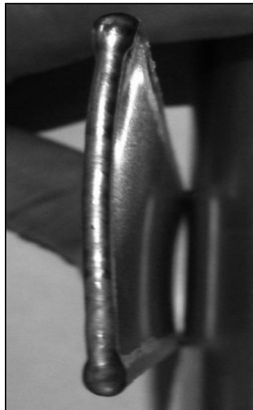
Figure 9. Curved plate type target with welded edges.
